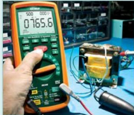
Measure the insulation resistance of transformer windings
