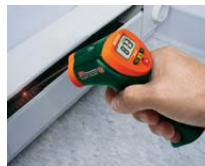
Test for temperature in heating systems
