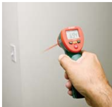
Check building for insufficient Insulation
