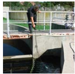
Sample testing with extension cable attached to meter
