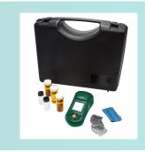
Meter comes complete with all the accessories to conveniently take measurements of both Free and Total Chlorine up to 3.50ppm with 0.01ppm resolution. The method used is adapted from USEPA Method 330.5 for waste water and Standard Method 4500-CI-G for drinking water.
