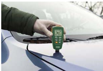
Measuring the thickness of automotive paint
