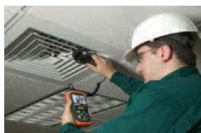
AN100 and AN200 used in HVAC applications measuring airflow from heating vents.
