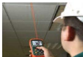
Model AN200 features built-in non-contact IR Thermometer to measure surface temperature that may be hard to reach
